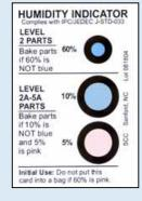
Blotting paper impregnated with cobaltous chloride. Based on ambient temperature of 75°F. Approx. 2.5% for each 10°F away from 75°F.
